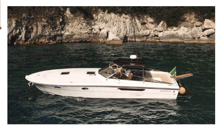
Type of Ship: Open Builder / Model: Itama / Itama 38 L.O.A. : 11,62 mt Beam: 3,77 mt Draft: 1,35 mt Tonnage: 11,30 ton Engines: 2 x 450 HP / FPT Speed: 32 kn (max.) - 25 kn (cr.) Max. 6 guests Internal cabin, WC, shower and sun awning Minibar with snacks and drinks included Music, towels and snorkeling gear
