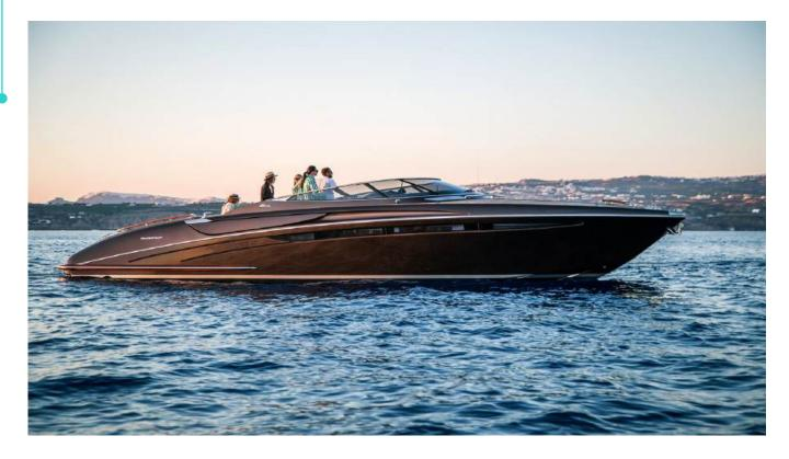
Type of Ship: OPEN Builder / Model: RIVA / RIVARAMA 44 L.O.A. : 13,30 mt Beam: 3,85 mt Draft: 1,03 mt Tonnage: 15,57 ton Engines: 2 x 800 HP / MAN Speed: 33 kn (max.) - 28 kn (cr.) Max. 6 guests Internal cabin, WC, shower and sun awning Minibar with snacks and drinks included Music, towels and snorkeling gear
