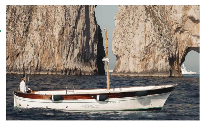
Type of Ship: Open Builder / Model: Fratelli Aprea / Aprea 7.80 L.O.A. : 7,85 mt Beam: 2,66 mt Draft: 0,70 mt Tonnage: 4,50 ton Engine: 1 x 150 HP / Yanmar Speed: 15 kn (max.) - 10 kn (cr.) Max. 6 guests Shower and sun awning Icebox with snacks and drinks included Music, towels and snorkeling gear
